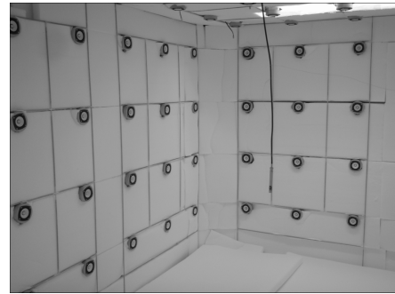
Figure 2: (a) Layout of the 157-channel irregular loudspeaker array. (b) 157-channel irregular loudspeaker array inside an anechoic room.
