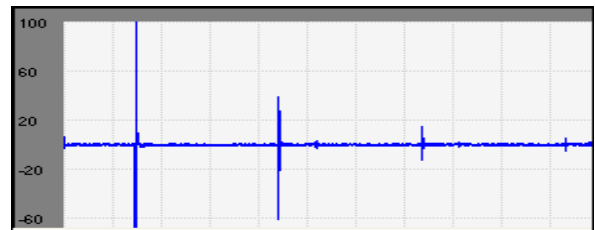
Figure 9: The transmitted pulse in water without the plate placed between the identical transducers. The vertical axis indicates the amplitude while the horizontal axis represents the elapsed time.
