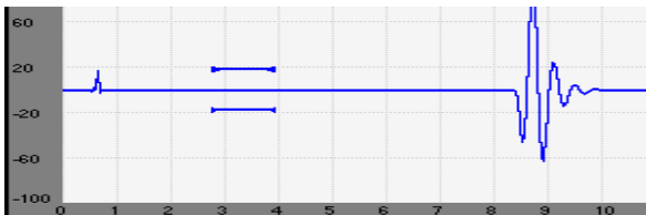
Figure 2: Experimentally measured initial pulse produced by the immersion transducer of 5MHz. The distance between the two probes without the plate is 7mm. The vertical axis indicates the amplitude while the horizontal axis represents the elapsed time.
