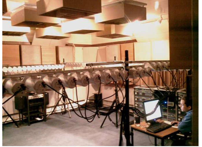
Figure 3. A prototype 128 channel Wave-field synthesis system at the University of Salford.
