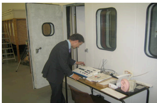
Source: (Zepidou, 2007) Figure 2. Environmental chamber with double layer doors and Amplivox audiometric equipment
