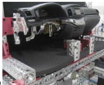
Figure 1. Test set-up for the BSR measurement of IP module with noise source measurement set-up(a), vibration system(b).
