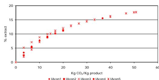
Figure 2. Repeatability. Kinetics of SFE tests with HPU.
