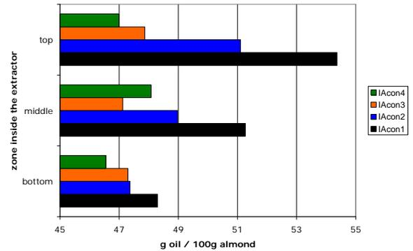
**Figure 9.** Almond oil content in different sections along time (SFE with HPU experiments)
