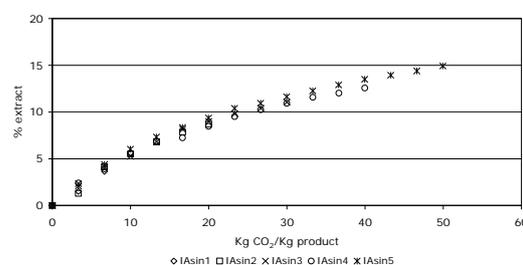
Figure 3. Repeatability. Kinetics of SFE tests without HPU.
