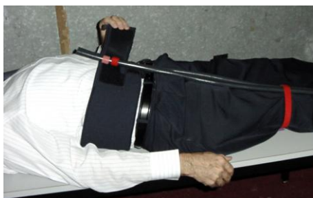
Figure 1 Tube immobilisation at the waist and leg reduced the problem of the ear-tip popping out of an ear.
