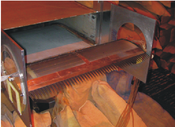
Figure 4. Picture of the NACA6512 airfoil in situ with serration \lambda_s/h_s = 0.6
