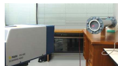
Photo.1 Scanning laser vibrometer (left side) and specimen through glass panel (right side)
