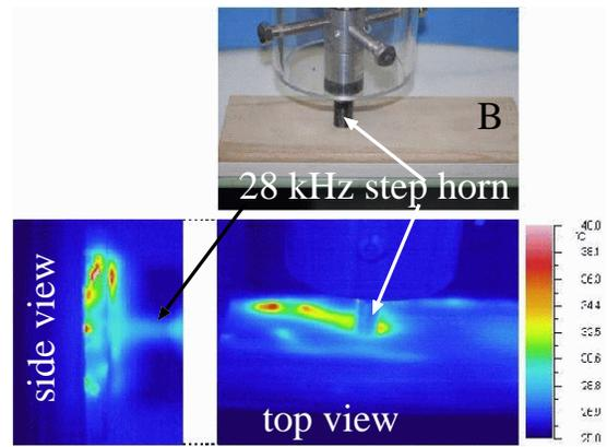
Figure 5: Temperature distribution of cedar board. The insect damage was clearly shown as the higher temperature.
