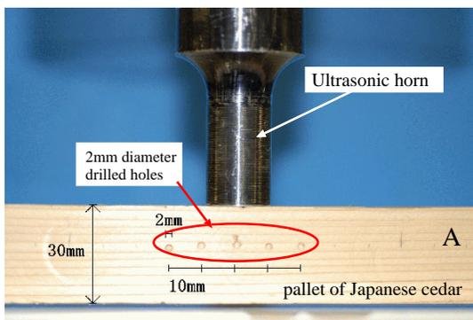
Figure 3: The horn connected on the side wall.
