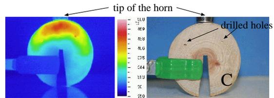
Figure 6: Sliced test piece of small Japanese cedar log having 2mm drilled holes(Right). Temperature distribution after 3 minutes(Left).
