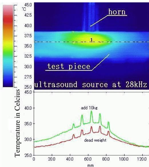
Figure 4: Temperature distribution on the surface of Japanese cedar. Ultrasound was irradiated for 3 minutes. Temperature around the holes got 4°C higher than the surrounding area.
