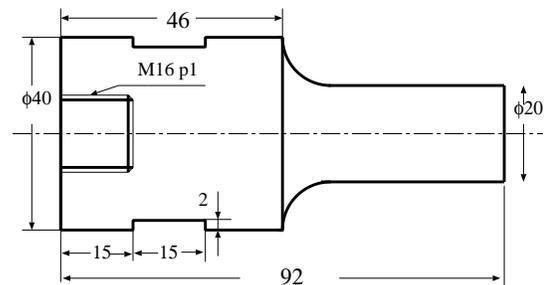
Figure 2: Design of a half wavelength step horn for 28 kHz vibration system.
