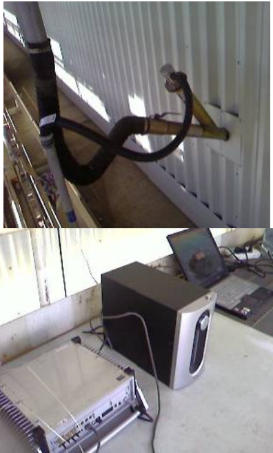
Fig.5 The microphone installed on the furnace and other experimental facilities
