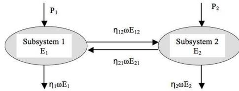
**Figure 1.** Power flow diagram of a two-subsystem SEA model
