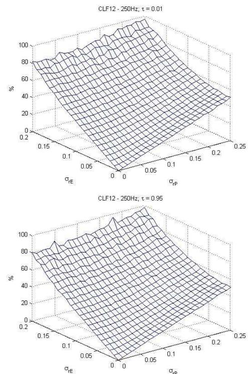
**Figure 3.** Relative uncertainty of the CLF values in the frequency band of 250Hz. Upper plot,  $\tau_{12} = 0.01$ ; lower plot,  $\tau_{12} = 0.95$ . Confidence level: 95 %
