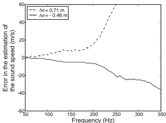
**Figure 4.** Error in the estimated sound speed in the sediment as a function of the frequency: sea state mismatch.  $SS_{ref}=3$  ( $\sigma_{ref}=0.35$  m),  $SS_i=4$  (i.e.  $\sigma_i=1.06$  m),  $SS_{ref}=3$  ( $\sigma_{ref}=0.71$  m),  $SS_i=2$  (i.e.  $\sigma_i=0.25$  m).
