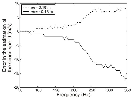
**Figure 3.** Error in the inverted sound speed in the sediment as a function of frequency: no sea state mismatch.  $SS_{ref}=3$  (i.e.  $\sigma_{ref}=0.35$  m and  $\sigma_{ref}=0.71$  m) and  $SS_i=3$  (i.e.  $\sigma_i=0.53$  m).
