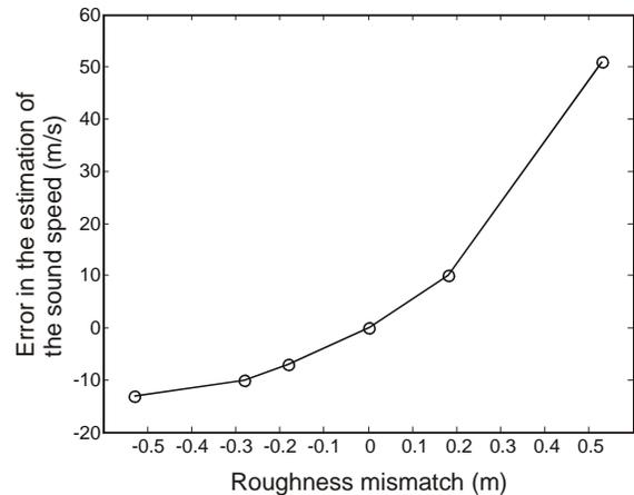
**Figure 2.** Error on the inverted sound speed in the sediment as a function of the roughness mismatch.
