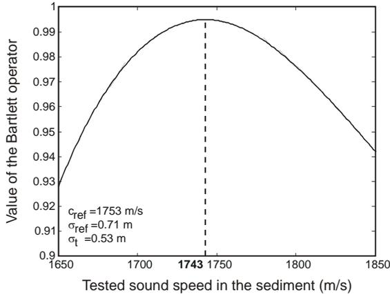
**Figure 1.** Value of the Bartlett operator as a function of the “tested” value of the sound speed in the sediment.
