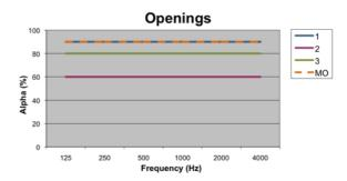
Figure 9e. Sound absorption of openings.
