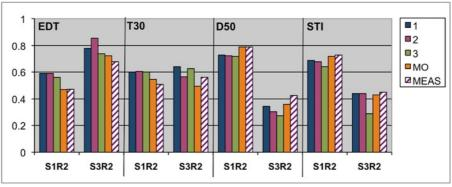
Figure 15. Comparison of all parameters EDT, T30 and D50 single number rating (average 500 – 1000 Hz) and STI with background noise.
