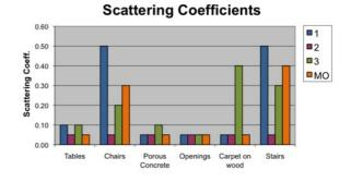
Figure 10. Scattering coefficients.
