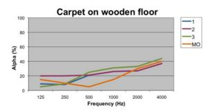
Figure 9c. Sound absorption of carpet on wooden floor.
