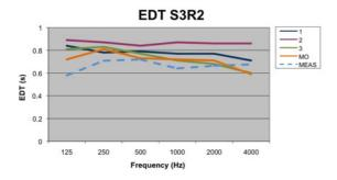
Figure 12b. EDT with source on floor above receiver.
