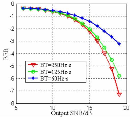
**Figure 5.** BER versus SNR and signal parameters
