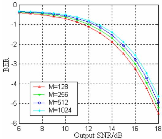
**Figure 4.** BER versus SNR and signal set size  $M$
