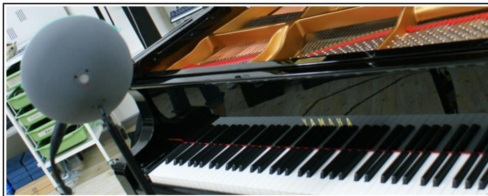
Figure 1: The sphere microphone, Schoeps KFM360, used to record pseudo-binaural signals for the given azimuth variation and each piano note automatically played by a MIDI controlled apparatus, DISKLAVIER. As pictured, the sphere microphone faces to +30^\circ from the center position. In addition, three cardioid microphones were placed near the hammers to be used for multichannel reproduction of piano sound. For the current study, the center cardioid microphone was used as a reference signal between the two channels of the sphere microphone.
