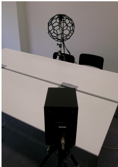
Figure 5: Picture of the impulse response measurement for voice filter
