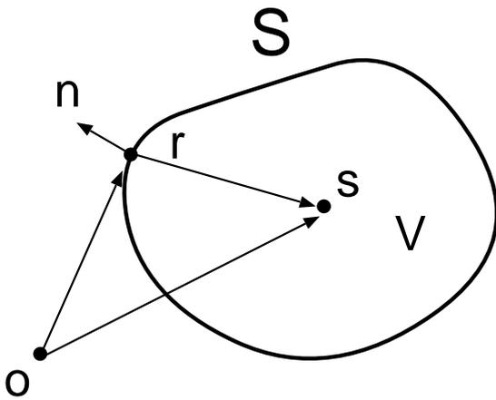
Figure 1: Region definition for the Kirchhoff-Helmholtz integral equation. The BoSC sound reproduction system is based on the KHIE. Volume  $V$  is completely bounded by surface  $S$ .  $\mathbf{n}$  is the outward normal vector.  $\mathbf{s}$  and  $\mathbf{r}$  are the evaluation point and observation point, respectively. The interior sound pressure  $p(\mathbf{s}, \omega)$  is fully determined by the sound pressure  $p(\mathbf{r}, \omega)$  and particle velocity  $v_n(\mathbf{r}, \omega)$ .
