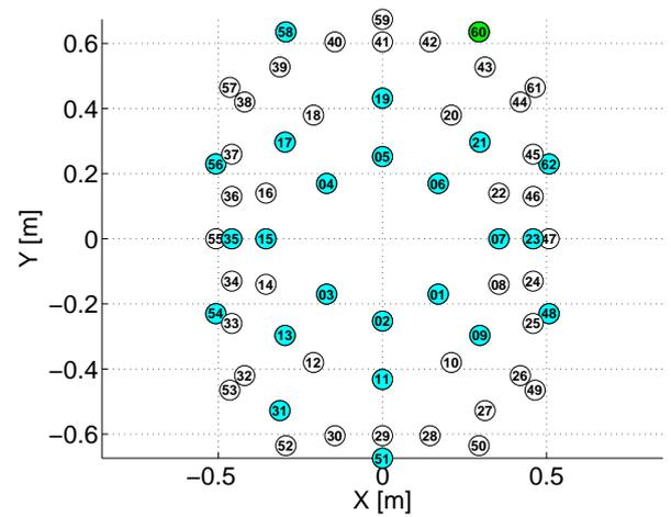
Figure 8: Selected loudspeaker location based on Gram-Schmidt orthogonalization. Loudspeaker #1 to #6 composes the first layer of the BoSC loudspeaker, #7 to #22 is the second, #23 to #46 is the third, and #47 to #62 is the fourth. Green point shows initially selected loudspeaker. Blue points show the selected loudspeakers as a result of the iteration based on Gram-Schmidt orthogonalization.
