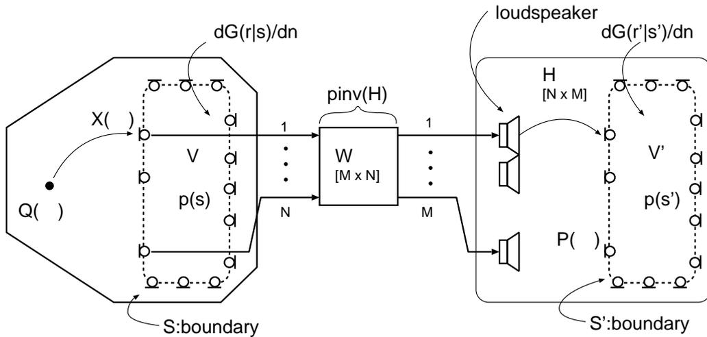
Figure 4: Inverse filter design for sound reproduction based on BoSC. The rooms depicted on the left and right side represent the primary sound field and reproduction room (listening room). The configuration of microphones on  $S'$  is congruous to it on  $S$ . As a consequence,  $V'$  and its bounding surface  $S'$  are congruous to  $V$  and its bounding surface  $S$ .
