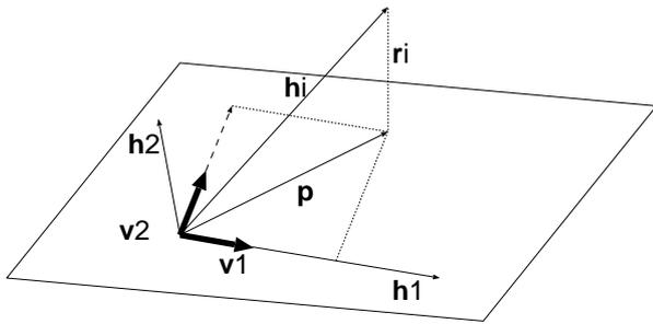
Figure 5: Column subspace of  $[\mathbf{H}(\omega)]$ . The subspace is spanned by  $\mathbf{h}_1$  and  $\mathbf{h}_2$ .  $\mathbf{p}$  denotes the projection of  $\mathbf{h}_i$  onto the subspace. For  $i = 3$ ,  $\mathbf{h}_i$  (third source) is determined so that the 2-norm of  $\mathbf{r}_i$  is maximized.
