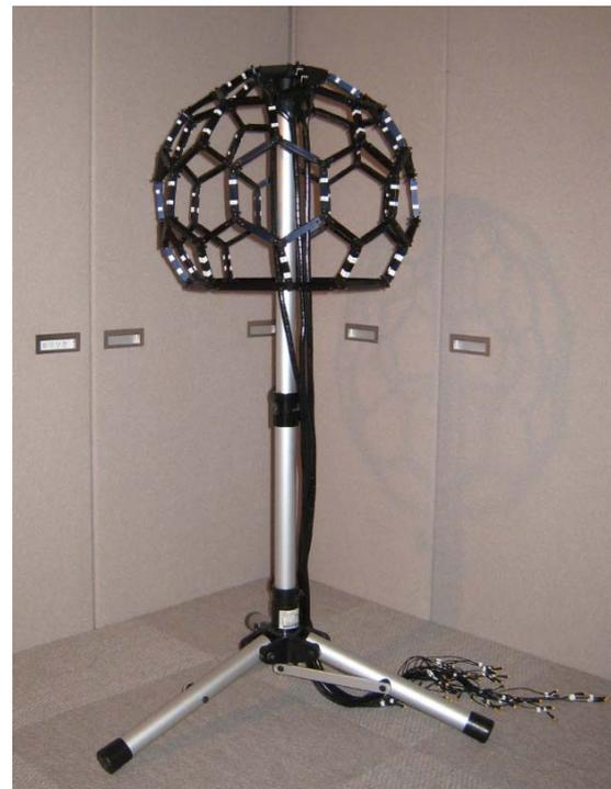
Figure 3: Microphone array for BoSC 3-D sound reproduction system. Microphone array is designed from the structure of C80 fullerene. Seventy omnidirectional microphones are put on each node.
