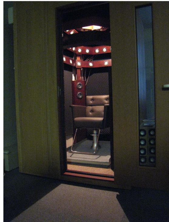
Figure 2: BoSC 3-D sound reproduction system. Loudspeaker array is installed in a soundproofed room with D-30 sound insulation level.
