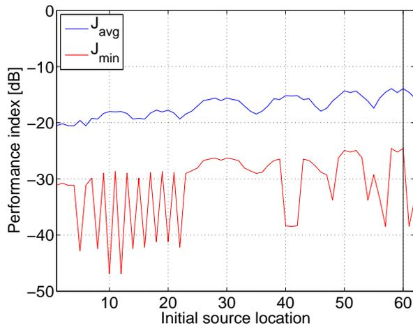
Figure 6: Performance indexes when 24 loudspeakers are selected. Blue line shows the  $J_{avg}$ , and red line shows the  $J_{min}$  for each initial selected loudspeaker location.
