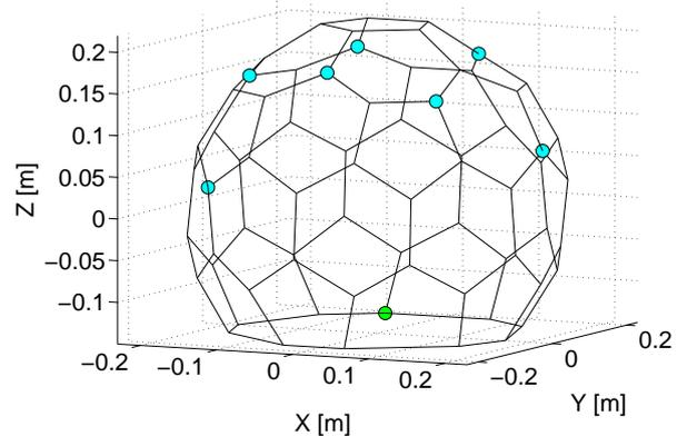
Figure 9: Selected microphone location based on Gram-Schmidt orthogonalization. Green point shows initially selected microphone. Blue points show the selected microphones.
