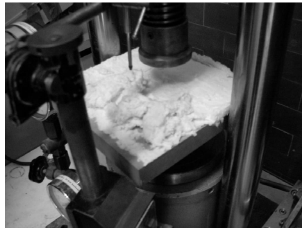
Figure 6. End of compressibility test for nano-composite layer. We can notice disgregation of the material
