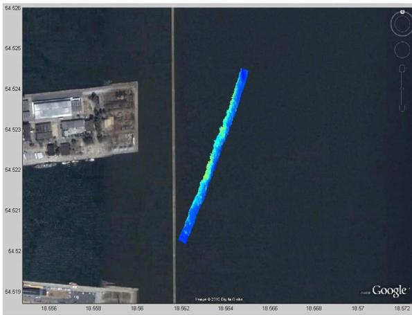
**Figure 7.** Imaging of seafloor surface from multibeam echosounder superimposed on satellite image from Google Earth
