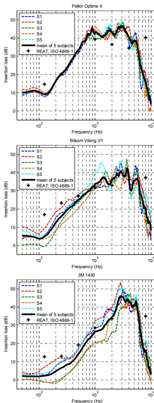
**Figure 1.** Insertion loss of a Peltor Optime II, Bilsom Viking V1, and a 3M 1430 earmuffs. Data measured with the MIRE technique on five subjects (dashed lines) and their mean (solid black line). Sound attenuation determined according to the REAT method (ISO 4869-1:1990) is shown by plus signs for a comparison (data declared by manufacturers)
