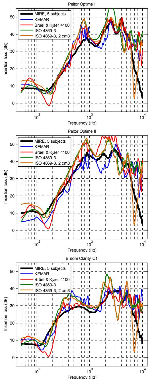
**Figure 3.** Insertion loss measured on the Kemar manikin, Brüel&Kjaer 4100 manikin, ISO 4869-3:2007 ATF, and the ATF equipped with the 2 cm<sup>3</sup> chamber compared to average MIRE data of five subjects (Peltor Optime I, Peltor Optime II, Bilsom Clarity C2 earmuffs)
