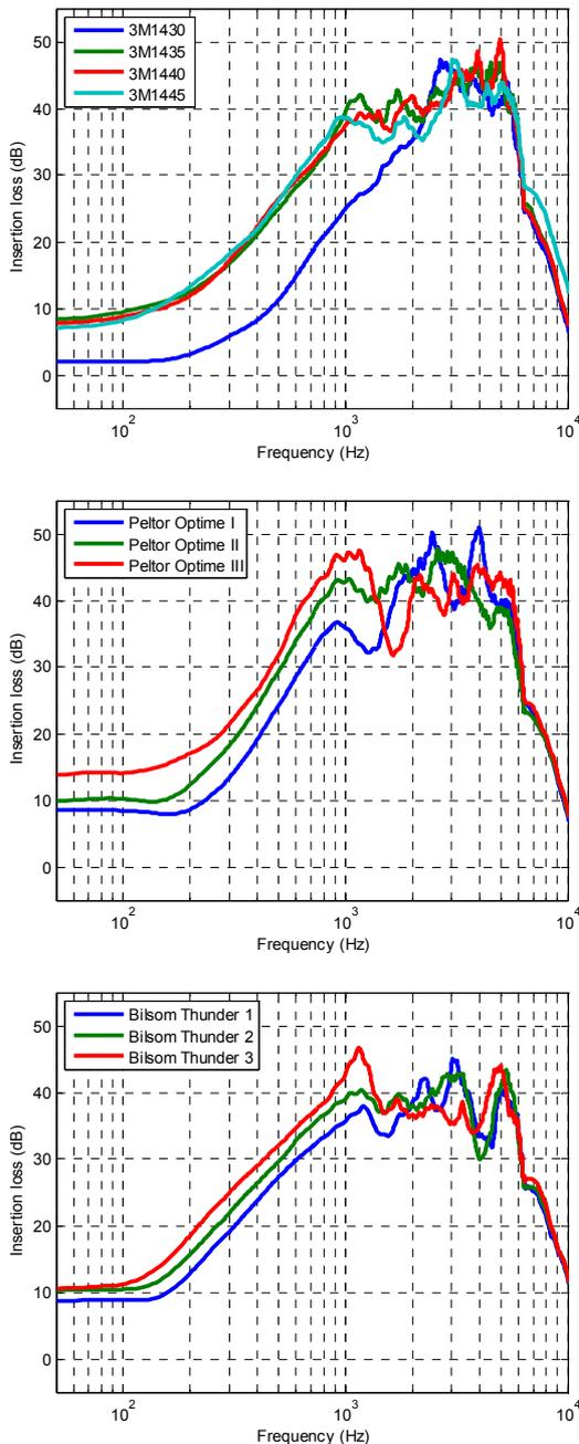
**Figure 2.** Insertion loss of the 3M (1430, 1435, 1440, and 1445), Peltor (Optime I, Optime II, and Optime III), and Bilsom (Thunder 1s, Thunder 2s, and Thunder 3s) earmuffs. MIRE method, average of 5 subjects
