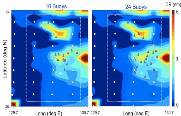
Figure 5. SCOUT optimized sensor locations (red triangles)
