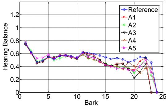
**Figure 6.** Hearing balance of different headphone with reference signal.
