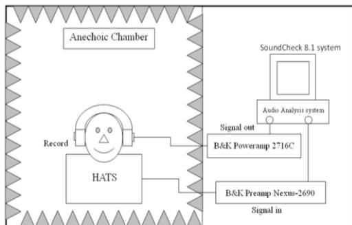
Figure 2. The schematic diagram for record headphones.
