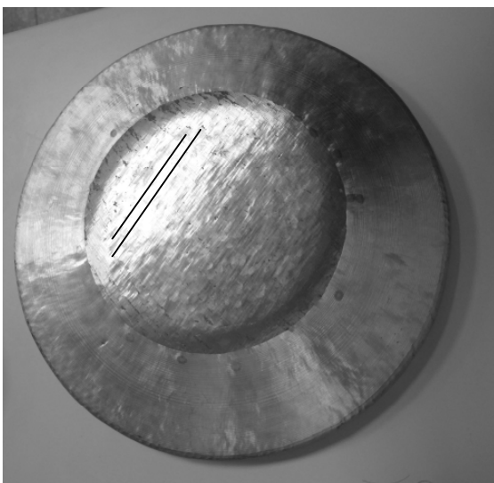
Figure 6. Striae on the flat surfaces of NX (top) and BL (bottom). The parallele lines indicate the direction of striae.
