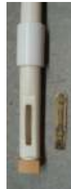
Figure 4. A harmonium type reed from an American reed organ coupled to a cylindrical pipe resonator
