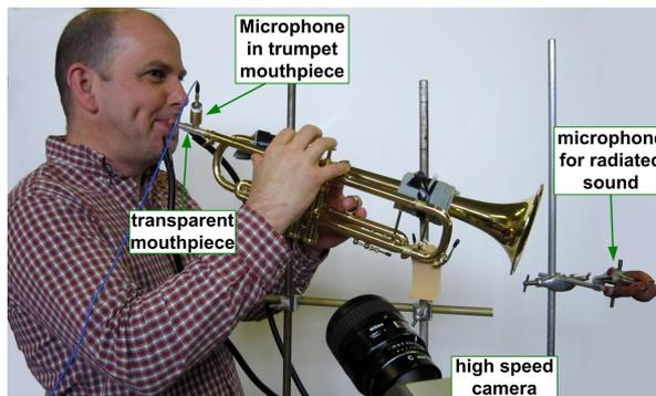
**Figure 7.** Experimental set-up for high speed filming
