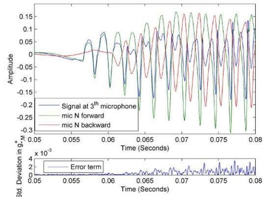
Figure 5. Wave separation for the 4<sup>th</sup> mode on trumpet
