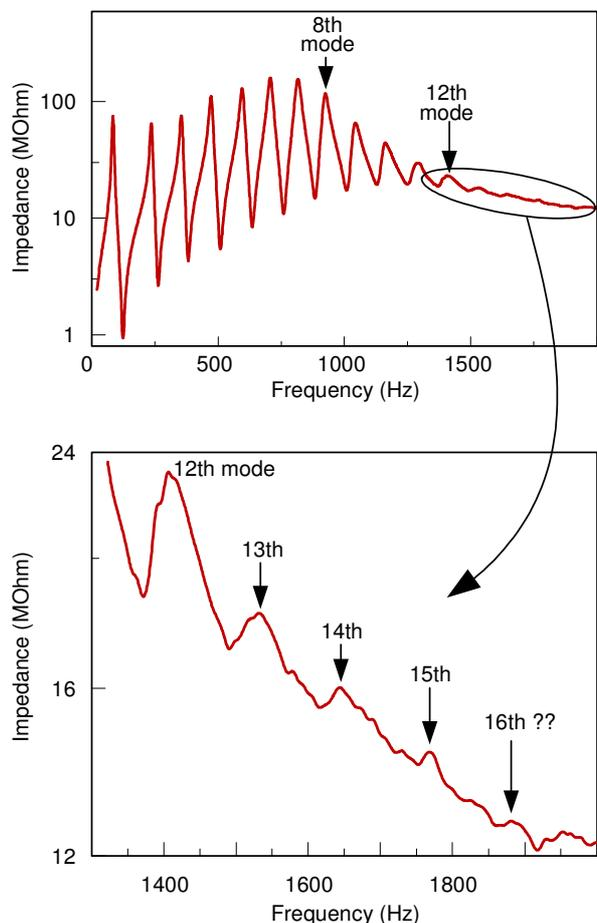
**Figure 1.** Input impedance of a modern trumpet and mouth-piece combination as used by specialist high players.
