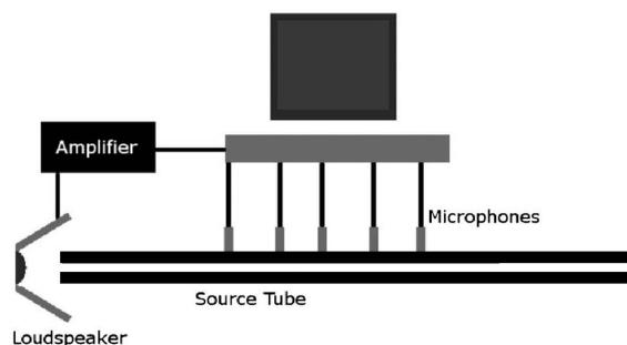
**Figure 2.** Schematic of calibration of the wave separation apparatus
