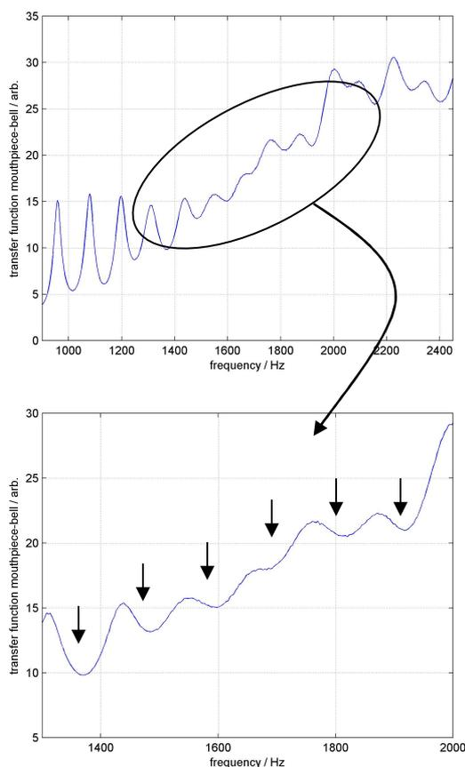
**Figure 6.** Transfer function between mouthpiece and outside bell for a modern trumpet and mouthpiece combination as used by specialist high players
