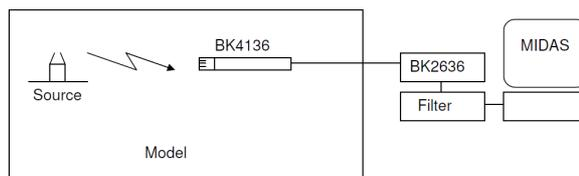
**Figure 13.** Setup for scale model measurements.
