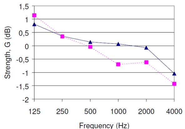
**Figure 5.** Average Strength, G. Blue triangles: Source on stage. Red squares: Source in pit.
