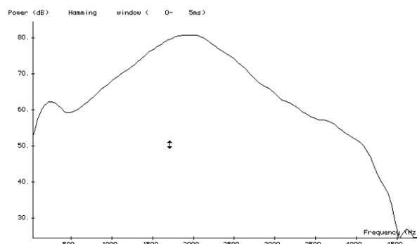
**Figure 14.** Frequency spectrum of the spark source (frequency axis is full scale).
