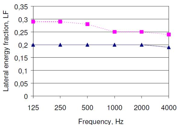
**Figure 7.** Average lateral energy fraction, LF. Blue triangles: Source on stage. Red squares: Source in pit.
