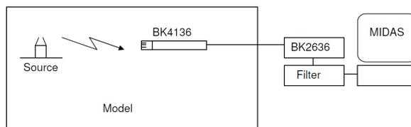
**Figure 13.** Setup for scale model measurements.
