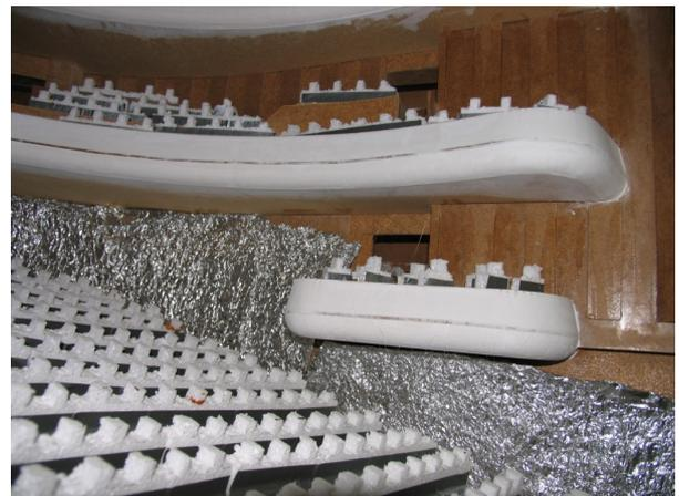
**Figure 29.** The scale model with sound diffusing treatment of the wall under the balcony.
