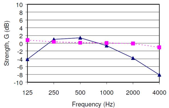
**Figure 23.** Average Strength, G with the source on stage. Blue triangles: Measured. Red squares: Simulated.
