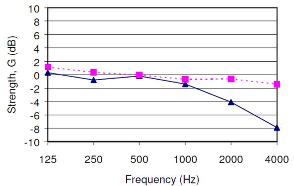
**Figure 24.** Average Strength, G with the source in the pit. Blue triangles: Measured. Red squares: Simulated.
