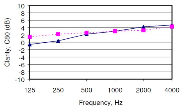
**Figure 25.** Average Clarity, C80 with the source on stage. Blue triangles: Measured. Red squares: Simulated.
