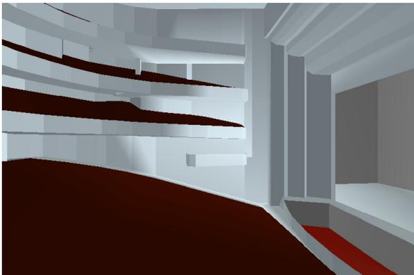
**Figure 2.** View into the computer model. Surface colours represent the different sound absorption characteristics.
