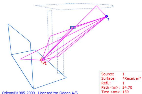
**Figure 30.** Example of an analysis in 3D of the reflection paths of early reflections.
