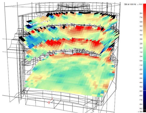
**Figure 10.** Grid response showing the Clarity C80 at 1 kHz. Source on stage.
