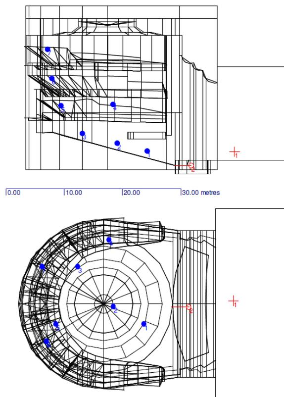
**Figure 1.** Section and plan of the digital model. The two source positions and the seven receiver positions are marked.
