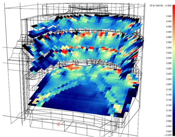
**Figure 11.** Grid response showing LF at 1 kHz. Source on stage.
