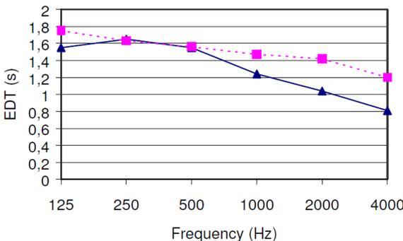
**Figure 22.** Average EDT with the source in the pit. Blue triangles: Measured. Red squares: Simulated.
