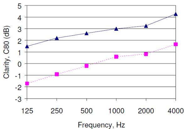
**Figure 6.** Average Clarity, C80. Blue triangles: Source on stage. Red squares: Source in pit.
