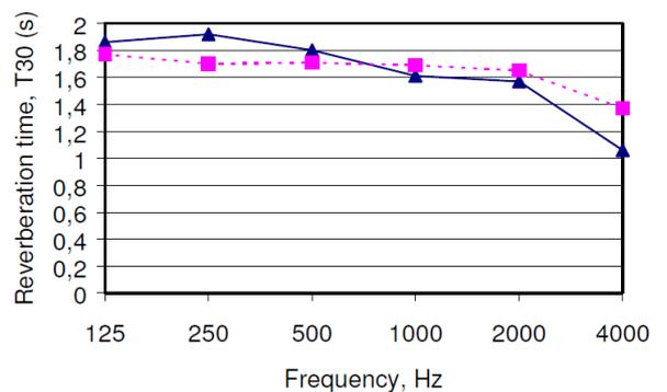
**Figure 19.** Reverberation time of the auditorium with the source on stage. Blue triangles: Measured. Red squares: Simulated.
