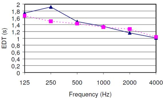
**Figure 21.** Average EDT with the source on stage. Blue triangles: Measured. Red squares: Simulated.
