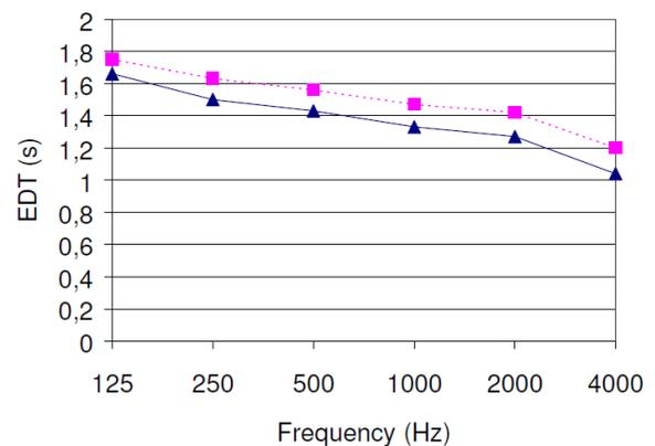
**Figure 4.** Average EDT. Blue triangles: Source on stage. Red squares: Source in pit.
