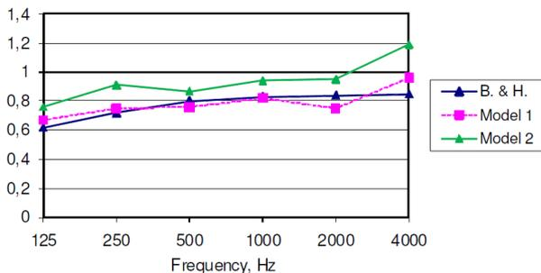
**Figure 17.** Absorption coefficient of audience for the 1:20 scale model compared to the Beranek & Hidaka data.
