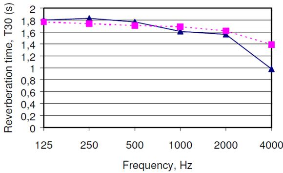
**Figure 20.** Reverberation time of the auditorium with the source in the pit. Blue triangles: Measured. Red squares: Simulated.
