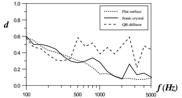
**Figure 4.** Diffusion coefficient versus frequency for a flat panel (dotted line), a sonic crystal with a flat surface backing (solid line) and a QR sound diffuser (dashed line). All surfaces are 3.6 m wide
