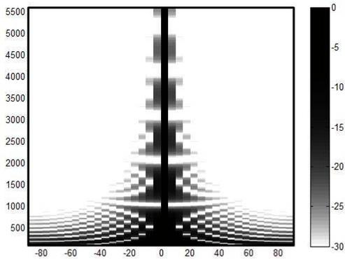
**Figure 2.** Flat surface (reference). The horizontal axis represents angle, the vertical axis is frequency. The gray scale corresponds to the relative intensity.
