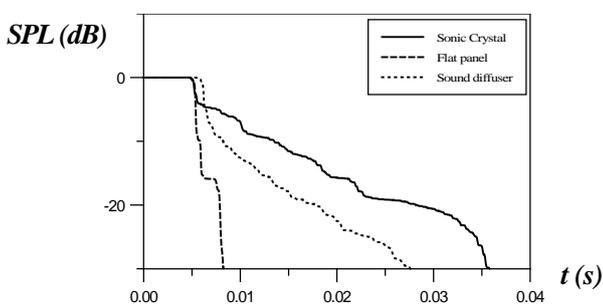
**Figure 8.** Normalized back-integrated time responses with Ricker wavelet excitation (only reflected sound) at 0 degrees versus time: Sonic Crystal (continuous line), flat panel (dashed line) and diffuser (dotted line).
