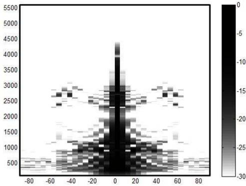
**Figure 3.** Sonic crystal. The horizontal axis represents angle, the vertical axis is frequency. The gray scale corresponds to the relative intensity.
