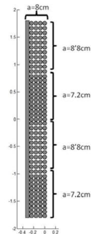
**Figure 5.** Second test specimen. The distance between elements in the  $y$  direction is abruptly changed from one zone to another.
