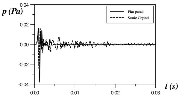
**Figure 7.** Sound pressure reflected at 0 degrees versus time: flat panel (continuous line), diffuser (dashed line)
