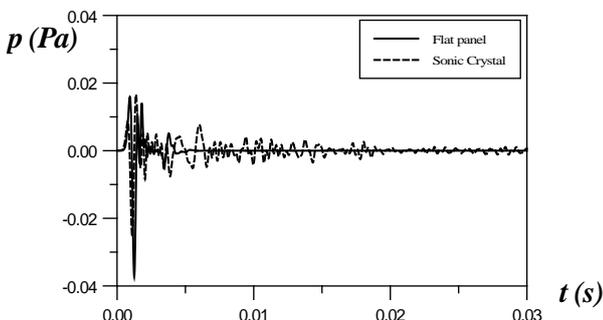
**Figure 7.** Sound pressure reflected at 0 degrees versus time: flat panel (continuous line), diffuser (dashed line)
