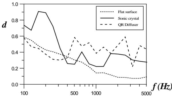
**Figure 6.** Diffusion coefficient versus frequency for a flat panel (dotted line), a sonic crystal with different distances between elements (solid line) and a QR sound diffuser (dashed line). All surfaces are 3.6 m wide
