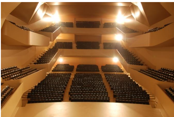
Figure 5. Picture of the 1:10 scale model hall
