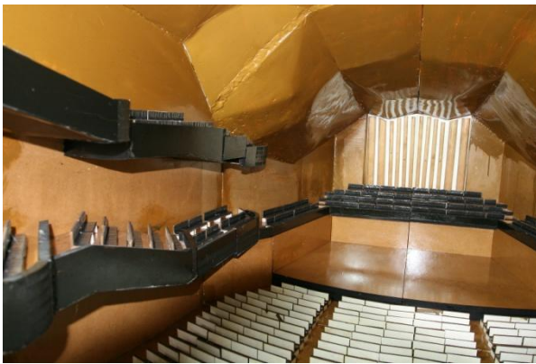
Figure 4. Picture of the 1:25 scale model hall without ceiling reflector
