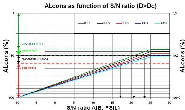
Figure 4.  $AL_{cons}$  as function of S/N for 5 values of RT.
