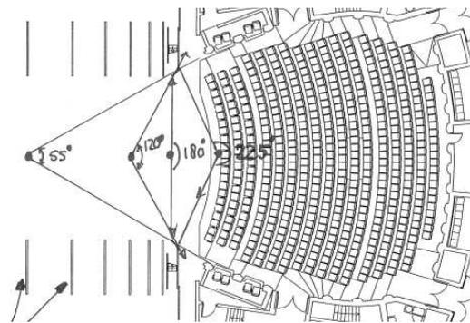
Figure 5. Ground level plan of theatre "de Spiegel" in Zwolle. The horizontal opening angle to the hall ( $\beta$ ) is indicated for 4 different source positions.
