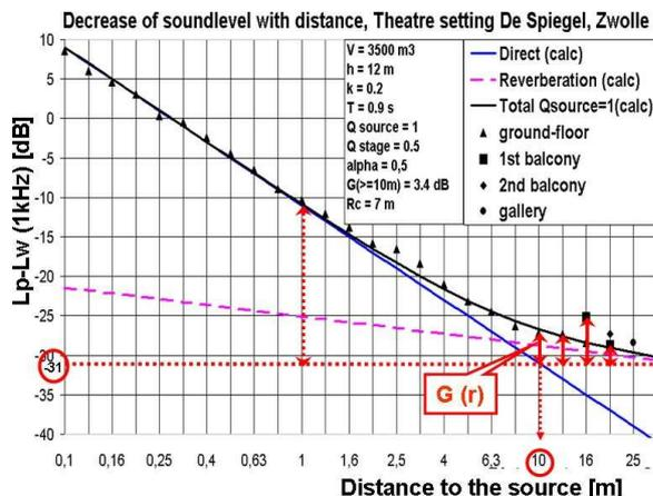
**Figure 13.** Decay with distance in theatre De Spiegel in Zwolle in theatre-mode, measured with an omni-directional source in the stage opening.
