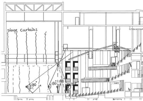
**Figure 6.** Cross-section of theatre “de Spiegel” in Zwolle. The vertical opening angle to the hall ( $\gamma$ ) is indicated for 4 different source positions.
