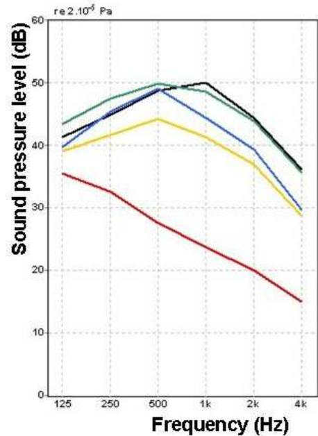
**Figure 14.** Measured sound level  $L_{eq}$  @row 12 during a theatre performance with non-reinforced speech in theatre “De Spiegel” in Zwolle. Background noise level (red line) 24 dB (PSIL). Speech level (2-3 min each) 47-52 dBL. Yellow 47 dBL. Resulting S/N=23 dB PSIL.
