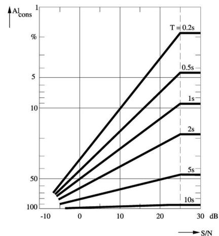
Figure 3.  $AL_{cons}$  as a function of S/N and  $T$  [1]
