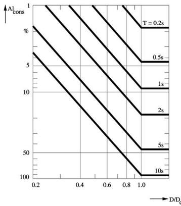
Figure 1.  $AL_{cons}$  as a function of  $D/D_c$  and  $T$  [1]
