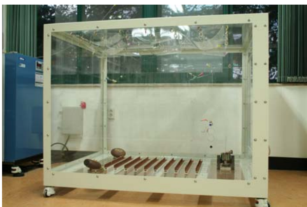
Figure 1. A 1/5 scale-model of the reverberation chamber (width: 1.2 m, length: 1.5 m, height: 1.1 m).
