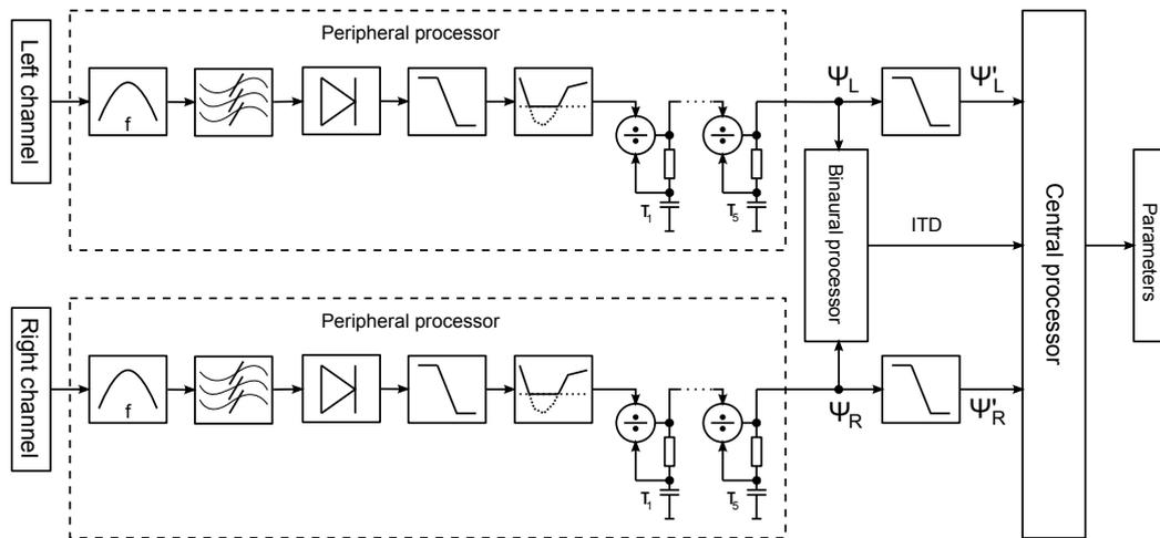
Figure 1: A schematic version of the binaural auditory model.
