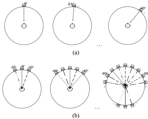
**Figure 2.** Examples of devised sound sources for the experiment: (a) point source at various directions, and (b) spanned decorrelated sources of various angular widths.
