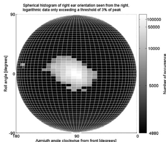
**Figure 1.** Spherical histogram of right ear position corresponding to the head orientation data collected during various acoustical evaluations. Each grid corresponds to 5° angular distance horizontally, and 2.5° vertically. View from the right hand side of the head (the nose is effectively half way up the right hand side of the sphere). Logarithmic data were used. Only data above a threshold of 3% of the peak are displayed.
