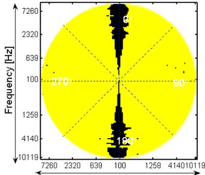
**Figure 7.** ITD difference for single point source, compared to the ITD JND, between the measurement at the target ear position and the ITD interpolated using the sinc function from those calculated at the adjacent microphone pairs ±5° apart (low-pass filtering applied to binaural signals in finding ITD).
