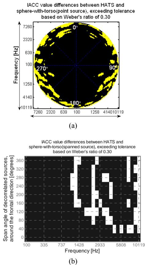
**Figure 4.** Plots of IACC differences between the HATS and the sphere with torso, compared to the JNDs: (a) for the simulated point source at various directions, and (b) for the simulated spanned sources with various angular widths. The bright area indicates that the difference exceeds the measurement tolerance, and the dark area indicates that the difference is within the tolerance.
