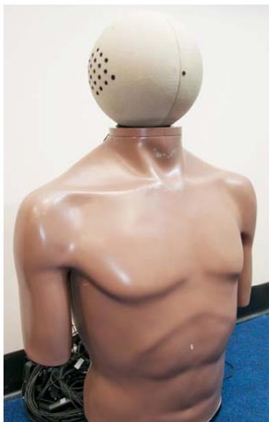
**Figure 11.** Developed prototype quasi-binaural signal capture system, based on the design suggested on Figure 10.
