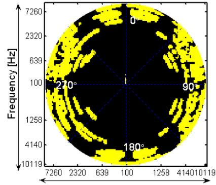
**Figure 9.** ITD difference for single point source, compared to the ITD JND, between the measurement at the target ear position with varying head orientation and the one linearly interpolated from those calculated at the microphone pairs ±5° apart (low-pass filtering not applied to binaural signals in finding ITD).
