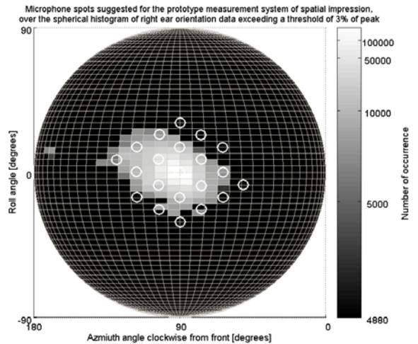
**Figure 10.** Suggested layout of microphones for the prototype measurement model of spatial impression incorporating head movements, drawn over the spherical histogram of Figure 1. The white circular marks indicate the suggested microphone spots. The small outstanding spot to the rear was excluded due to practicality and the small number of occurrences.
