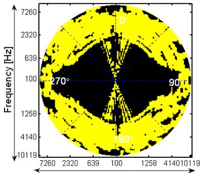
**Figure 8.** ITD difference for single point source, compared to the ITD JND, between the measurement at the target ear position and the ITD calculated from the linearly interpolated binaural signals at the adjacent microphone pairs +12.5° and -10° apart (low-pass filtering applied to binaural signals in finding ITD).
