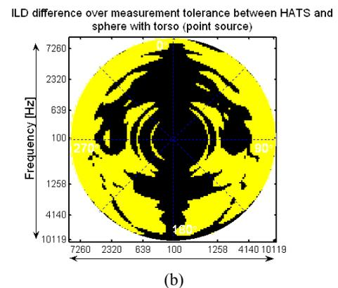
**Figure 3.** Plots of ITD and ILD differences between the HATS and the sphere on a torso, compared to their JNDs as the measurement tolerances. The bright area inside the disc indicates that the difference exceeds the JND for the corresponding source direction and frequency band, and the dark area indicates that the difference is within the JND.
