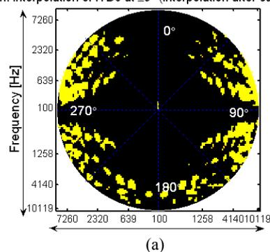
ITD difference over tolerance, calculated for single source at  $0^\circ$ , between measurements at target ear positions and lin. interpolation of ITDs at  $\pm 12.5^\circ$  and  $-10^\circ$  (interpolation after calc.)
