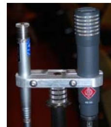
Figure 3. Microphones in custom mic-stand used for the impulse response measurements.
