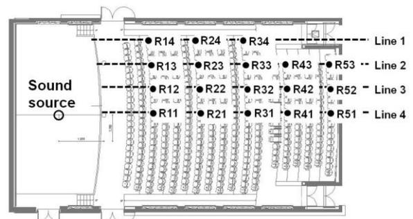
Figure 2. Source and receiver positions
