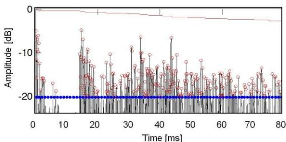
**Figure 3.** Calculation of *Number of peaks* in the measured impulse response
