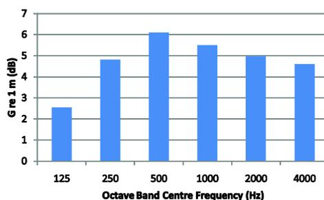
**Figure 6.** Measured  $G$ , referenced to 1 m instead of 10 m, measured at a distance of 1 m from the dodecahedral loudspeaker at the sweet spot in the untreated room.
