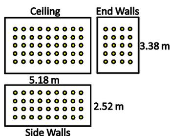
**Figure 2.** Layout of the loudspeakers on the ceiling and walls.
