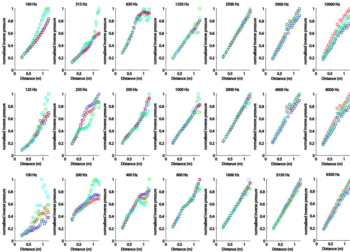
**Figure 7.** Inverse of pressure (the square root of integrated squared pressure) along the four horizontal traverses in 1/3-octave bands. Bands from 100 Hz – 3.15 kHz use the dodecahedral source, and bands from 4 kHz – 10 kHz use the pipe loudspeaker. The four traverses are indicated by four colours.
