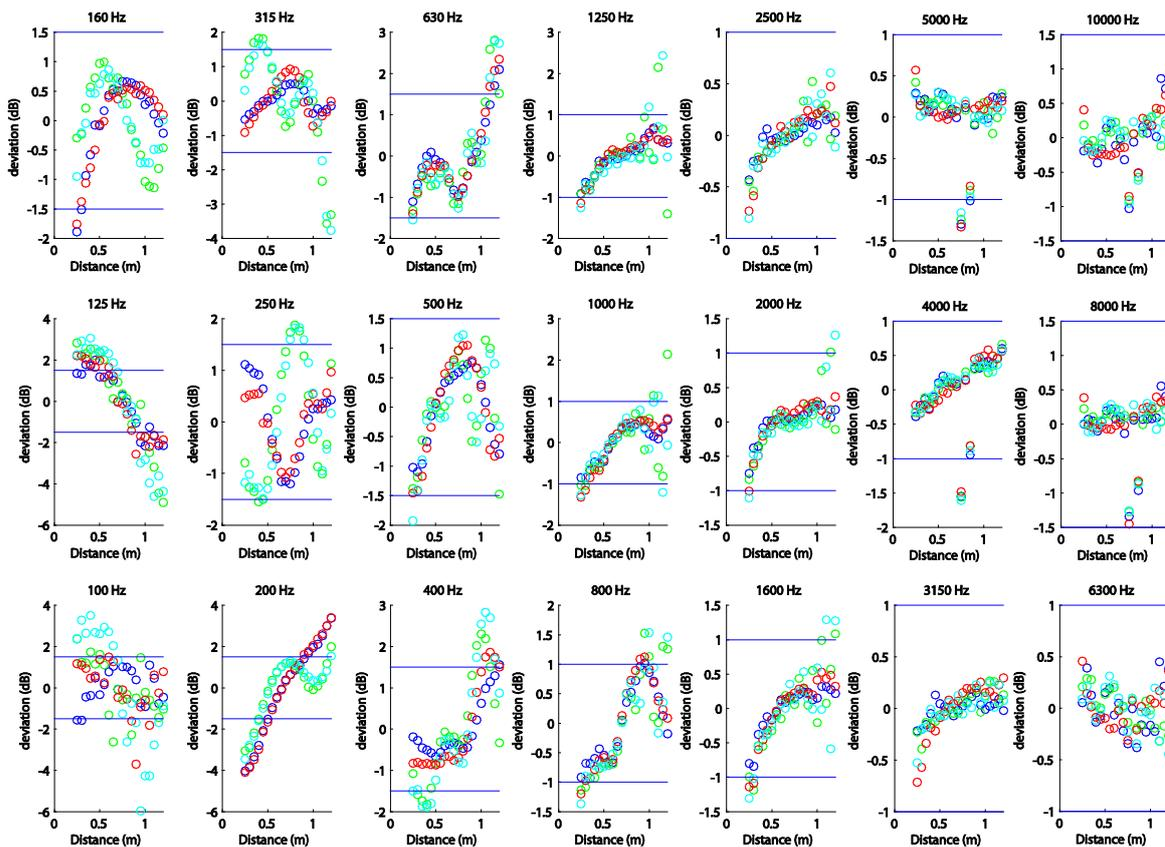
**Figure 8.** Deviations from the inverse-square law for 1/3-octave bands from 100 Hz-10 kHz (measured as described previously). The four traverses are indicated by four colours. The horizontal lines indicate the allowable limits for anechoic room qualification.
