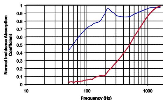
**Figure 3.** Normal incidence sound absorption coefficients of one 50 mm layer of the PET sound absorbing batt (no air gap, shown in red), and of the room lining as it was typically applied (four layers of 50 mm PET fibrous absorber distributed over a 300 mm depth, shown in blue).
