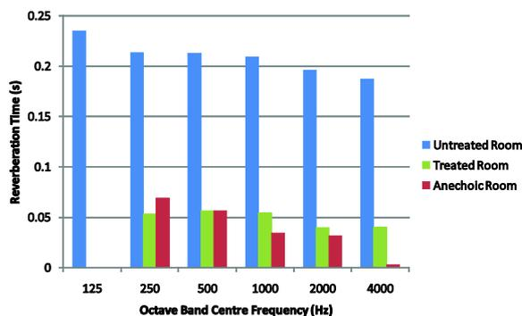
**Figure 5.** Measured reverberation time of the room prior to the installation of sound absorptive lining, after the installation of absorptive lining, and the apparent reverberation time of the measurement loudspeaker measured in a large anechoic room. In the latter two cases, reliable values could not be derived for the 125 Hz octave band.
