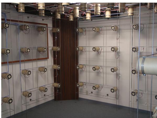
**Figure 1.** Photograph of the room prior to acoustic treatment, showing a fibre-glass panel on the left wall, an edge absorber, and the cylindrical loudspeakers.
