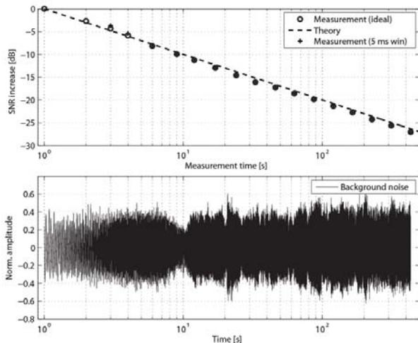
**Figure 6.** Theoretical and practical achievable SNR gain (top) based on measured background noise (bottom) transformed by inverse filters of sweeps of different length.
