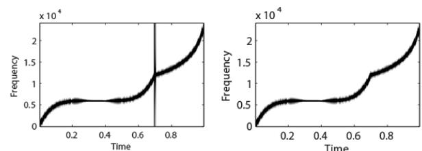
**Figure 1.** Spectrograms of a sine sweep consisting of 2 segments concatenated. Left: unaligned. Right: phase aligned. The audible click (vertical line in the left figure) is mitigated if phase-alignment is conducted.
