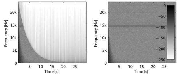
**Figure 5.** Measurement examples with a 30-second exponential sweep using measurement length  $T$  (left) and  $2T$  (right). Colors denote magnitude in dBFS. Truncated signals (left) will introduce frequency-dependent double slope energy decay curves because the noise is truncated.
