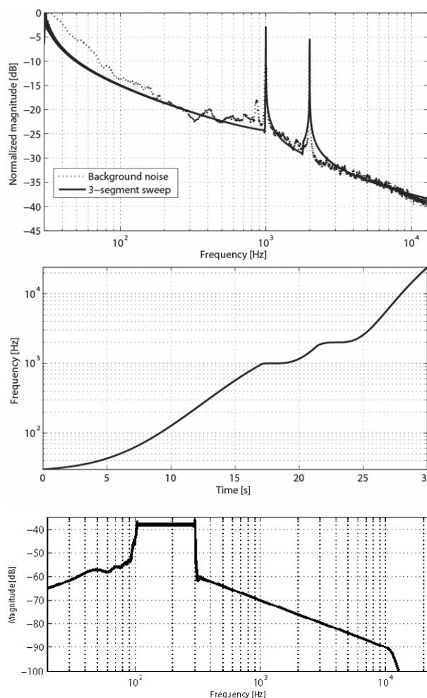
**Figure 8.** Overall magnitude spectrum and spectrogram of the 3-segment sine sweep optimized for the twin harmonic noise (top) and spectrum of the signal optimized for the 100-300 Hz band background noise. In the latter case, half-windowing attenuates the signal above 10 kHz.
