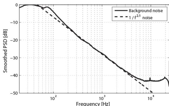
**Figure 7.** Average smoothed power spectral density of observed background noises (including equipment noise) in 23 different halls, using 2-second noise samples of 1933 different measurements (solid), and a robust linear regression fit (dashed) on the obtained result.  $\beta = 2.1$  means that the background noise is similar to a red noise.
