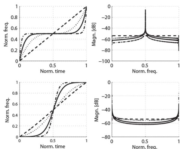
**Figure 3.** Frequency focus and notch with monomial and sigmoid sweeplets; left: spectrogram, right: spectrum. Top: monomial power sweeplet,  $d = \omega_2/2$ ; dashed  $p = 1$ , dotted  $p = 3$ , solid  $p = 7$ , dotted dashed  $p = 21$ . Bottom: sigmoid sweeplet with dashed  $d$  and  $c$  jointly increasing.
