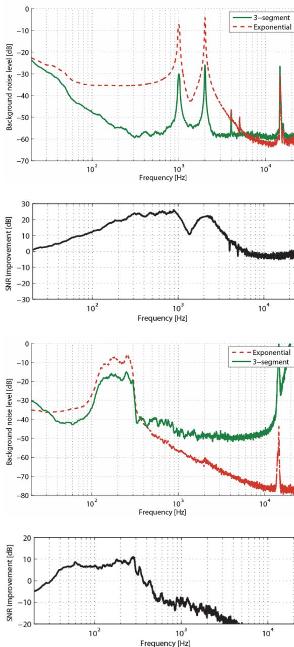
**Figure 9.** Relative background noise and SNR improvement in the impulse response in the presence of a two-harmonic noise in addition to the room noise (top two); and in the presence of additional 100-300 Hz band noise (bottom two). Optimization was achieved in these examples in the desired frequency range at the expense of SNR reduction in the other frequency ranges.
