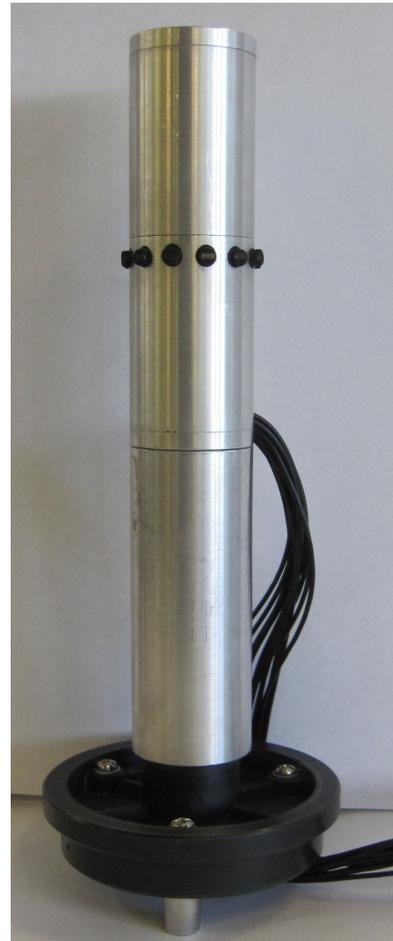
Figure 3: This figure shows a photo of the 12 sensor cylindrical microphone array used for the room measurements.
