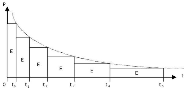
Figure 4: Energy decays exponentially. Each sample contains the same amount of energy. The instants of time defining the samples are denoted  $t_0, t_1, t_2$ , etc. The vertical axis is acoustic power,  $P$ , and the horizontal axis is time,  $t$ . Energy  $E = \int_{t_{n-1}}^{t_n} P(t) dt \approx P(t_n)(t_n - t_{n-1})$  is constant.
