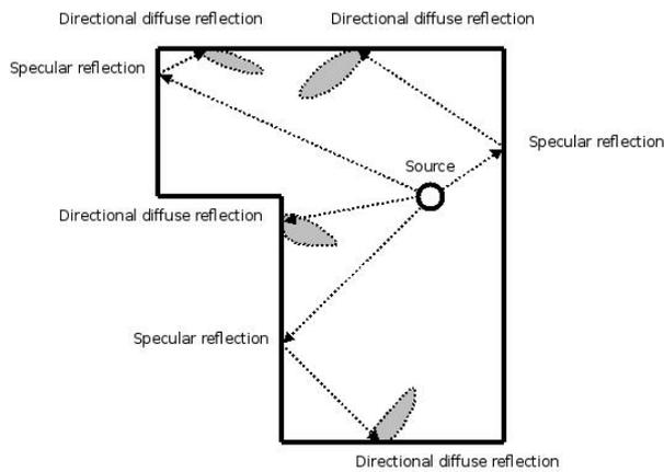
Figure 5: In the hybrid model, early reflections are modelled as specular reflection with a beam tracing method and later reflections are modelled as directional diffuse reflections with the acoustic radiance transfer method. Also pure directional diffuse reflection paths are included as well as low order pure specular reflections.
