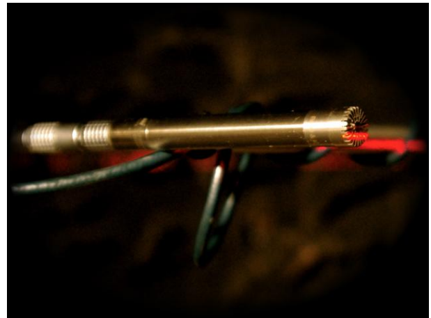
(b) The centers of the two microphones are in plane with the axis of the top rod.
