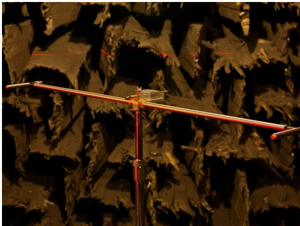
(a) The stand is made from steel rods with polished surface making laser-aided alignment easy.
