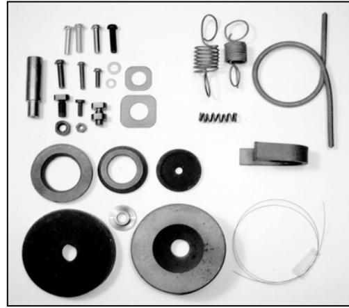
Fig. 2. Photos of the mechanical parts, thin sheet and wires made from M2052 damping alloy.
