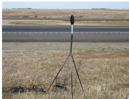
Figure 2. Noise measurement study equipment setup at the Highway 11, Saskatchewan, Canada
