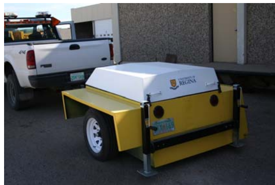
Figure 4. Custom-build trailer for traffic noise measurement study using CPX method
