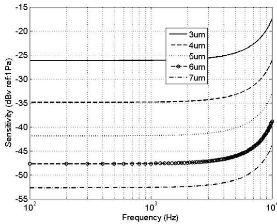
Fig.4 The effects of the air gap distance on the sensitivity
