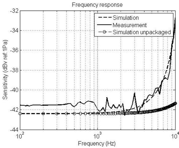
Fig.2 MEMS microphone simulation and measurement.
