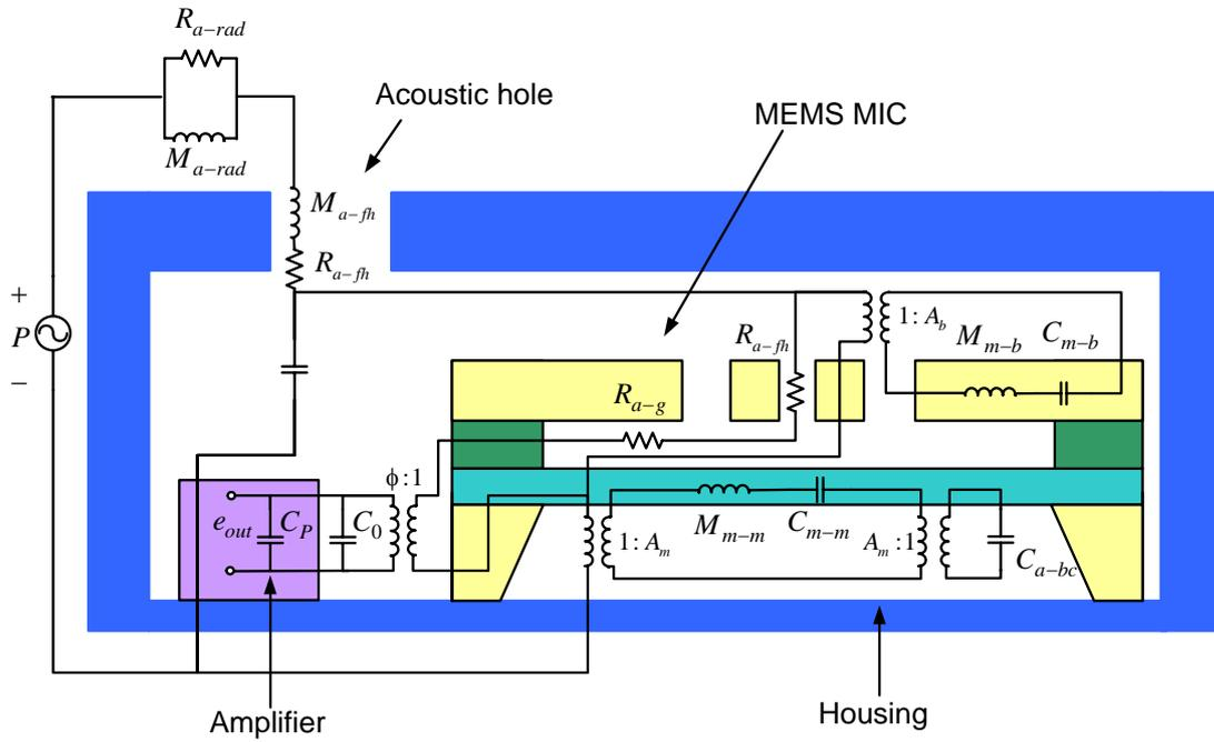
Fig.1 Equivalent circuit for the packaged MEMS condenser microphone.
