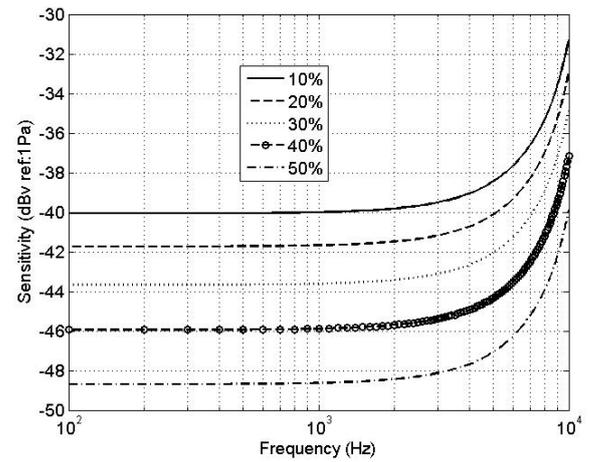
Fig.5 The influence of the acoustical holes on the performed backplate.
