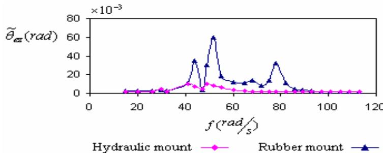
Figure 9. Variation of steady state amplitude of engine rotation about “z” axis versus frequency of road excitation.
