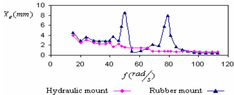
Figure 5. Variation of steady state amplitude of engine displacement in “x” direction versus frequency of road excitation.
