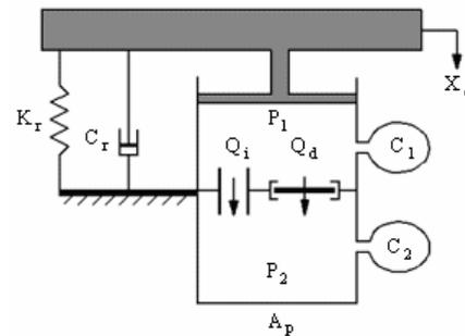
Figure 2. Lumped parameter model [6].
