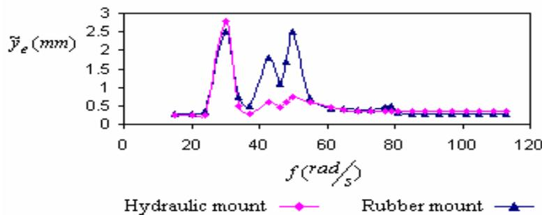
Figure 6. Variation of steady state amplitude of engine displacement in “y” direction versus frequency of road excitation.
