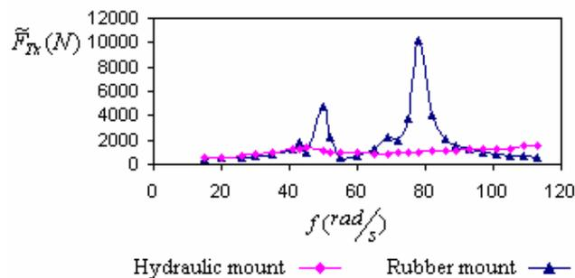
Figure 10. Variation of steady state amplitude of transmitted force to the body by engine mounts in “x” direction versus frequency of road excitation.
