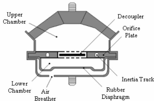
Figure 1. Cross-section of hydraulic engine mount [6].
