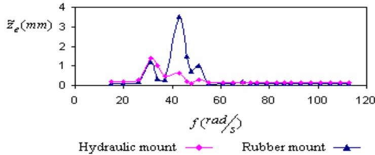
Figure 7. Variation of steady state amplitude of engine displacement in “z” direction versus frequency of road excitation.
