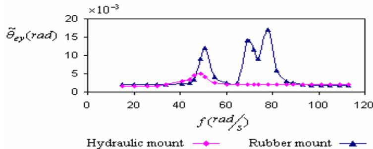
Figure 8. Variation of steady state amplitude of engine rotation about “y” axis versus frequency of road excitation.
