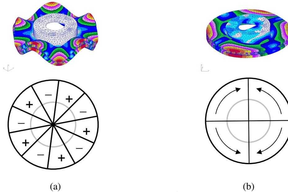
Figure 3. (a) Bending mode with 5 nodal diameters, (b) 2<sup>nd</sup> order tangential in-plane compression mode
