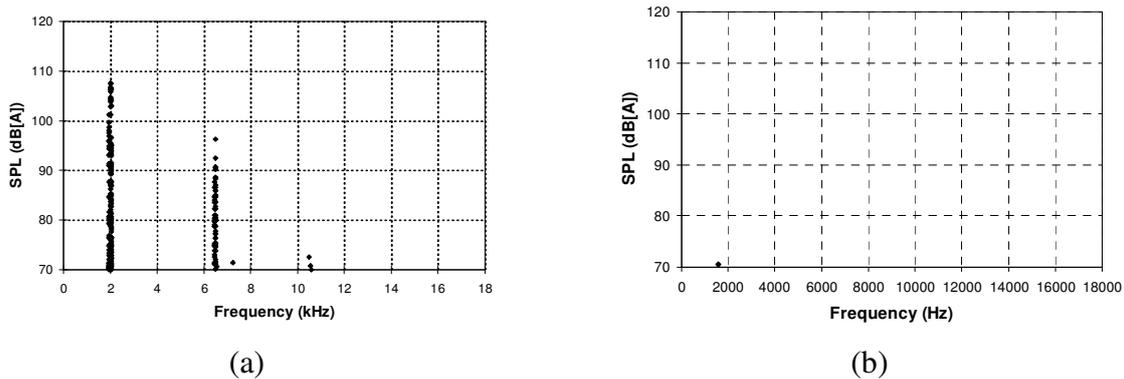
Figure 8. Procedure B OTV (a) Noise performance with OTV caliper, corrected rotor, (b) Final OTV performance with modified chamfer and rotor
