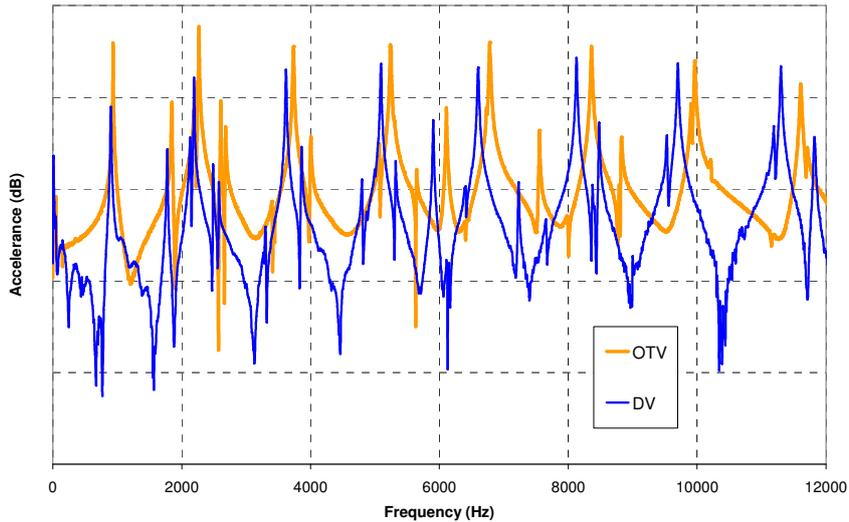
Figure 7. OTV and DV brake rotor frequency response functions.
