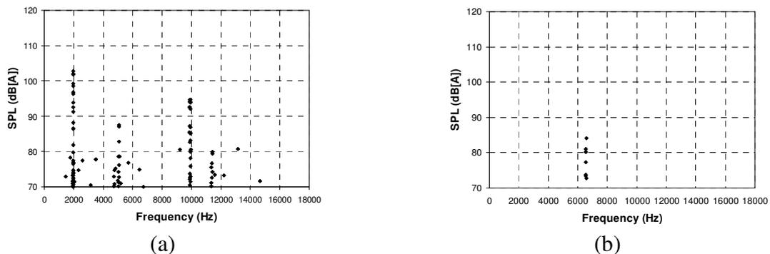
Figure 5. (a) Initial DV noise performance, (b) Final DV noise performance with modified pad chamfer and backplate shim material change.
