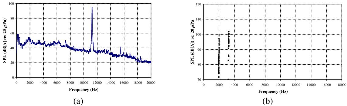
Figure 1. (a) Typical brake squeal spectrum (b) SPL vs Frequency for noise events over 70 dB(A)
