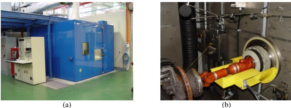
Figure 2. (a) Industrial brake noise dynamometer and environmental system. (b) Internal brake fixture
