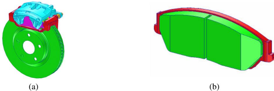
Figure 4. (a) Example brake system used in the case study. (b) Brake pad with 20mm chamfer
