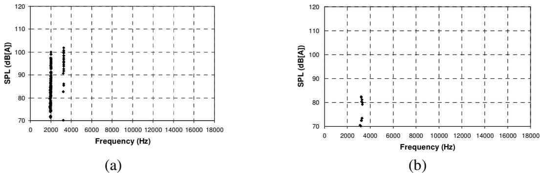
Figure 6. Procedure A OTV (a) Initial performance, (b) Noise with corrected rotor composition
