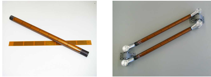
Figure 2. Active rods for the TRIGLIDE: The left side depicts the embedded piezo-actuator and the finished rod, the right side shows a complete link including electrical connections of the actuators.
