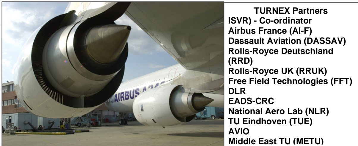
Figure 1: Bypass exhaust nozzle and the hot core exhaust nozzle of a Rolls-Royce Trent 500 on an Airbus A340 and TURNEX Consortium Partners
