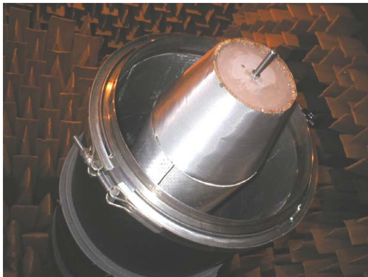
Figure 6: ISVR/RR No-flow rig with Inner & Outer Lined Bypass and Lined Afterbody Configuration
