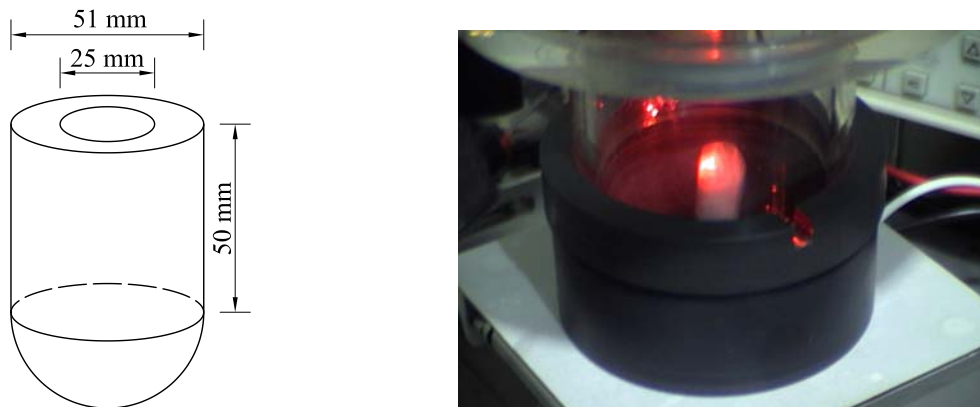
Figure 1. Diagram (left) and a picture (right) of the cavity used for the experiments. The latter shows the moment at which the oscillating sphere blocks a laser beam implemented to detect the time when the sphere was at the top of its movement.
