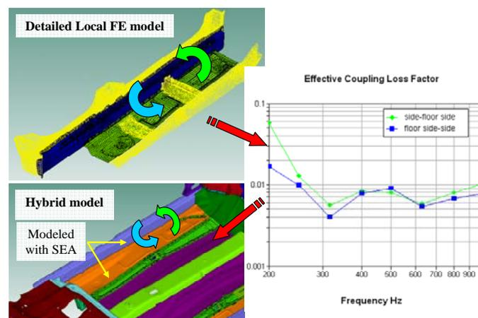
Figure 3. Characterization of SEA coupling loss factors through local EFM models – floor side/rail.
