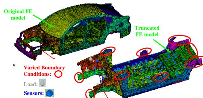
Figure 5. Initial FE model of BIW car and truncated model used for numerical validation of the Hybrid model.
