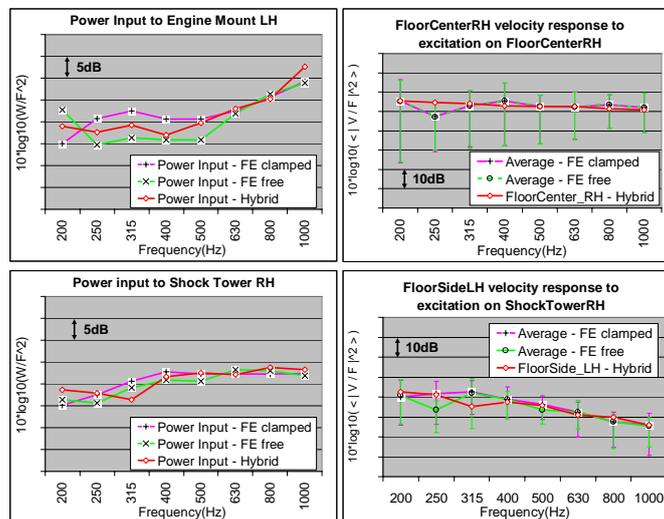
Figure 6. Example numerical validation results – Left: Power Input, Right: average velocity response in some SEA regions.
