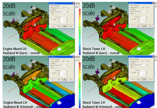
Figure 8. Noise contribution analysis, Top/bottom: bare/trimmed floor, Left/right: engine mount LHS / shock tower LH loading.
