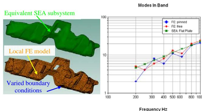
Figure 2. Characterization of subsystems for SEA – toeboard.
