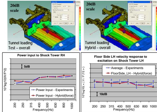
Figure 7. Experimental validations results. Top: measured and predicted contour maps of velocity response to rain-on-the-roof loading of the tunnel region. Bottom: power input and velocity response to point force loading on the shock tower.
