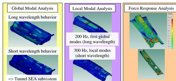
Figure 1. Verification of the subsystem partitioning: tunnel region.
