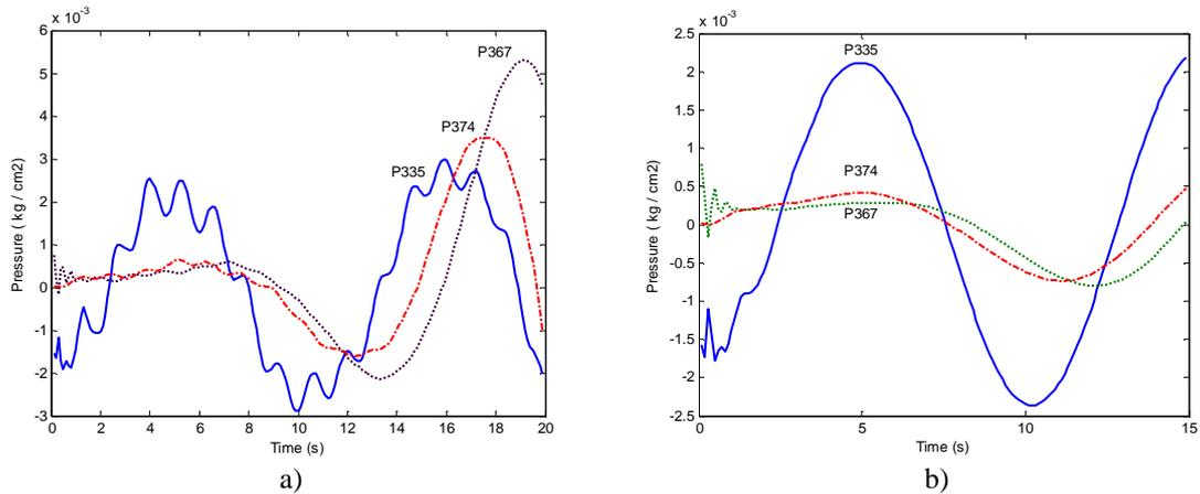
Figure 6. Dynamic pressure response curves at the selected points on the internal tank wall at frequency  $f = 0.1\text{Hz}$ : mode damping factor a) 0.05 ; b) 0.2 .
