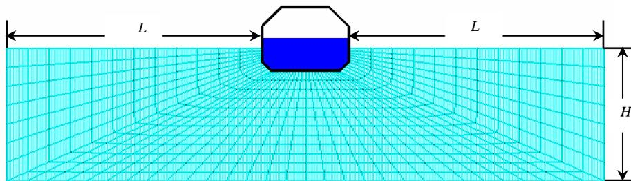
Figure 3. The finite element idealization of an internal liquid – LNG tank – external water system.
