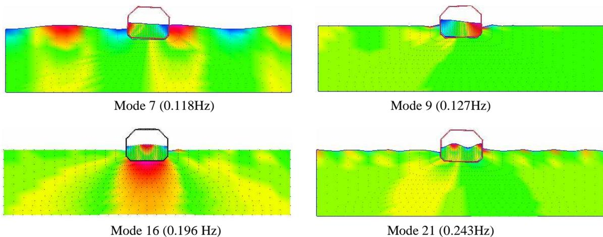
Figure 4. Selected modes of internal liquid-tank-external water interaction system.
