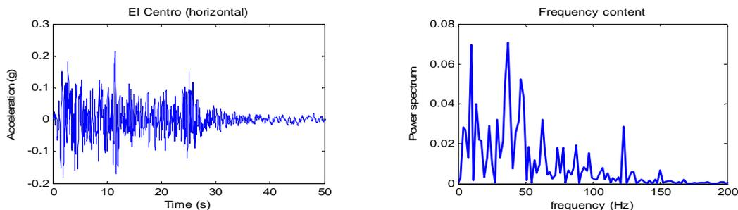
Figure 9. El Centro East-West earthquake data [21]: a) time history; b) power spectrum.
