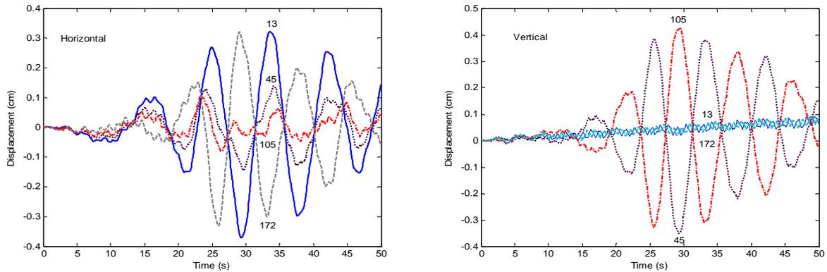
Figure 10. Horizontal and vertical displacement responses at the chosen points of the system excited by the earthquake ground motion.
