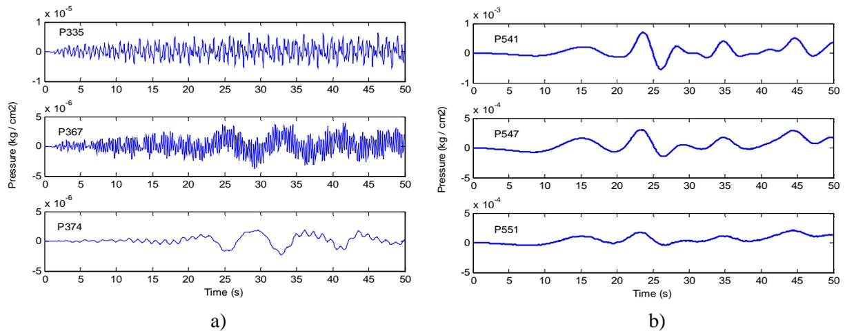
Figure 11. The dynamic pressure responses at selected points on internal a) and external b) tank walls due to the earthquake ground motion excitation.
