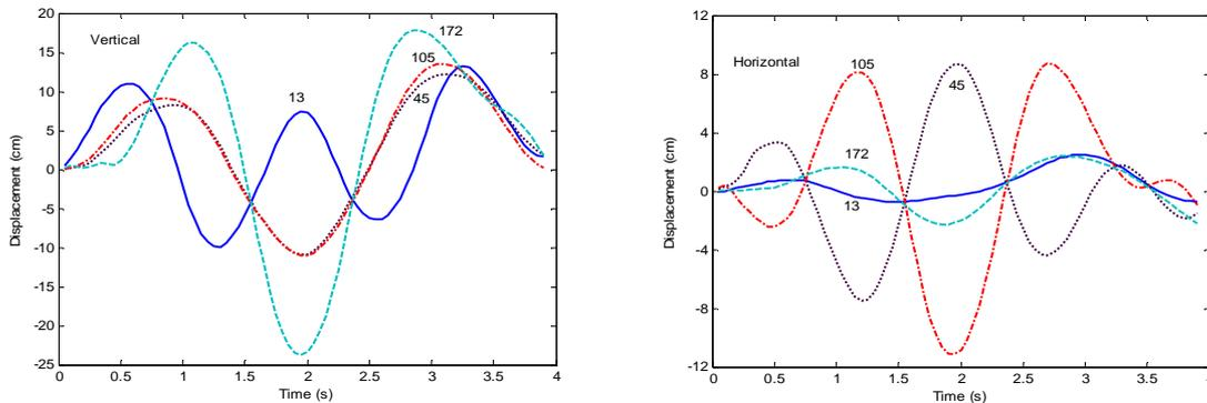
Figure 7. Vertical and horizontal displacement responses at chosen points of the tank ( $f = 0.5$  Hz).
