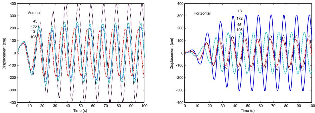
Figure 5. Vertical and horizontal displacement responses at chosen points of the tank ( $f = 0.1\text{Hz}$ ).
