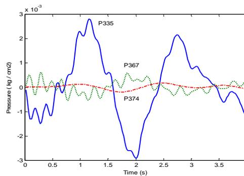
Figure 8. Pressure responses at selected points on internal tank wall ( $f = 0.5$ Hz).
