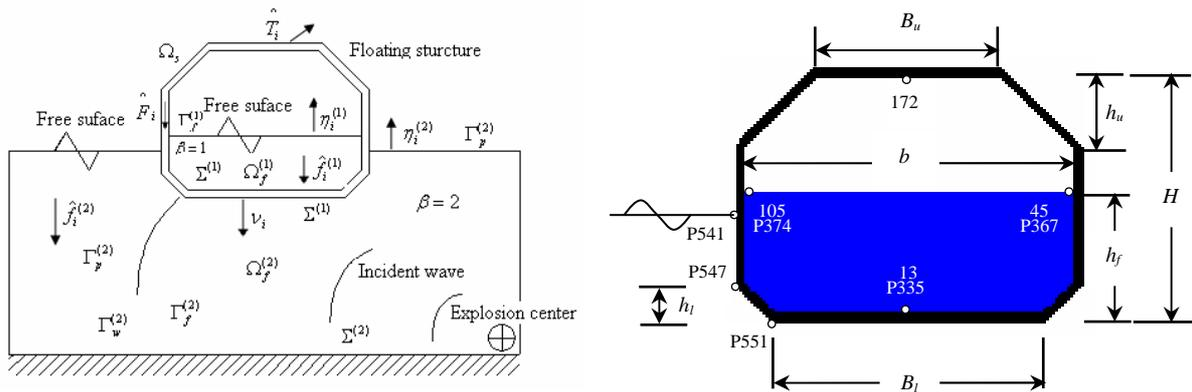
Figure 1. A general LNG ship-water interaction system. Figure 2. Geometrical size of a filled tank.
